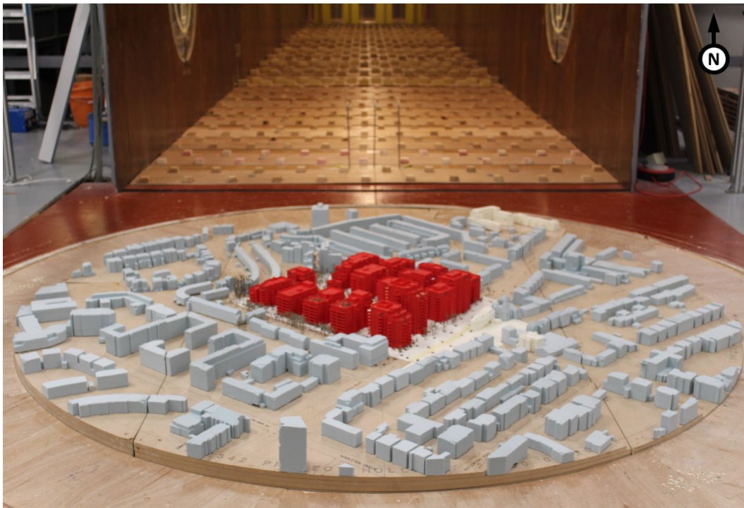
Figure 13: The Development with existing and proposed landscaping and cumulative schemes plus proposed mitigation measures (Configuration 6) – View in the Wind Tunnel (from the south)
