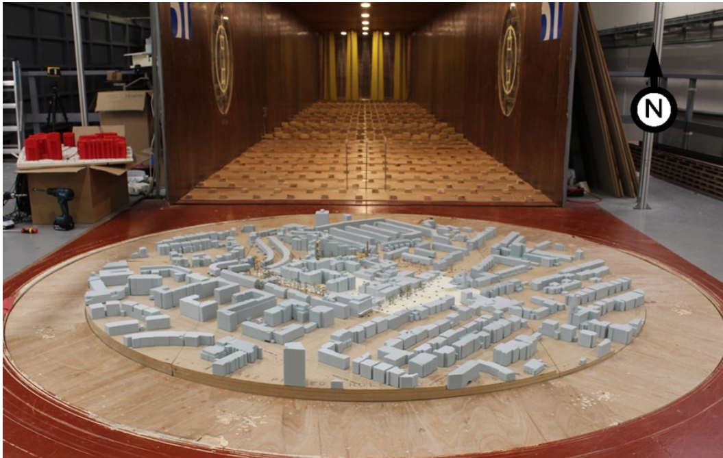
Figure 3: Existing Site with existing landscaping and existing surrounding buildings (Configuration 1) – View in the Wind Tunnel (from the south)
