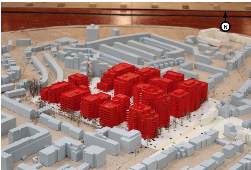
Figure 10: The Development with existing landscaping and Cumulative Schemes (Configuration 4) – View in the Wind Tunnel (from the south)
