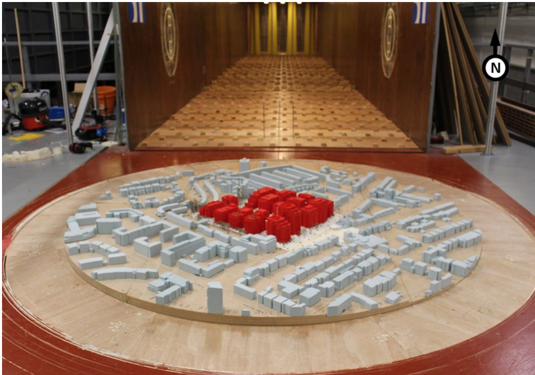
Figure 7: The Development with existing and proposed landscaping and existing surrounding buildings (Configuration 3) – View in the Wind Tunnel (from the south)
