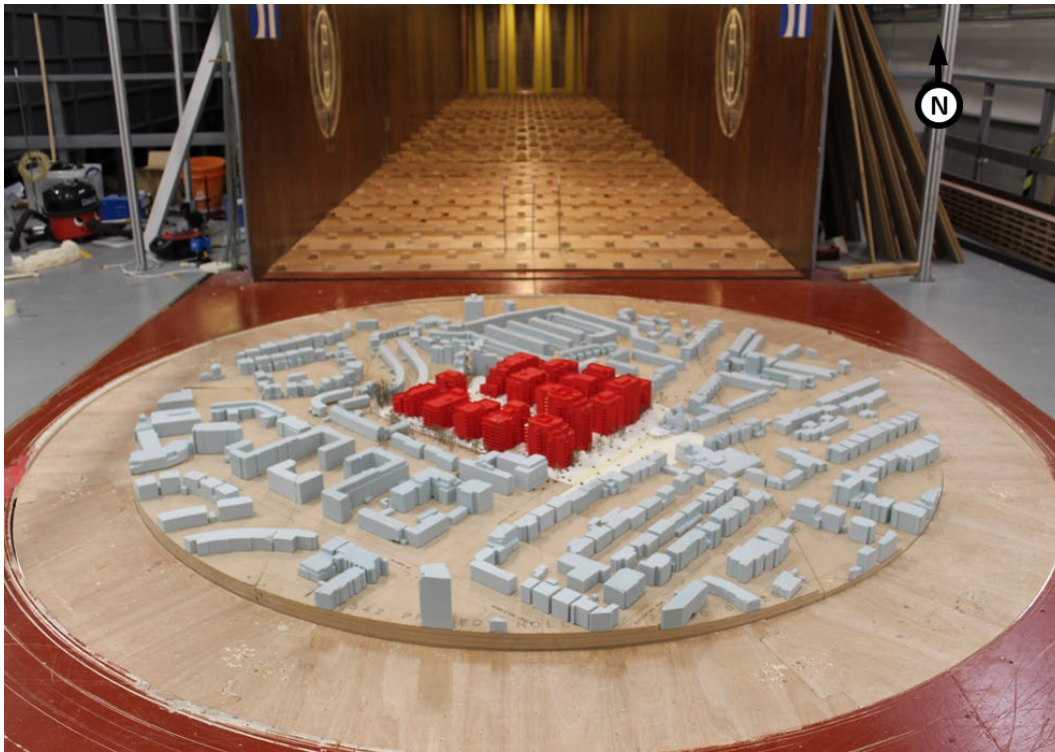
Figure 5: The Development with existing landscaping and existing surrounding (Configuration 2) – View in the Wind Tunnel (from the south)
