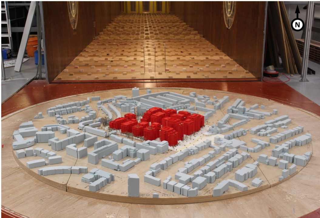
Figure 11: The Development with existing and proposed landscaping and existing surrounding buildings plus proposed mitigation measures (Configuration 5) – View in the Wind Tunnel (from the south)
