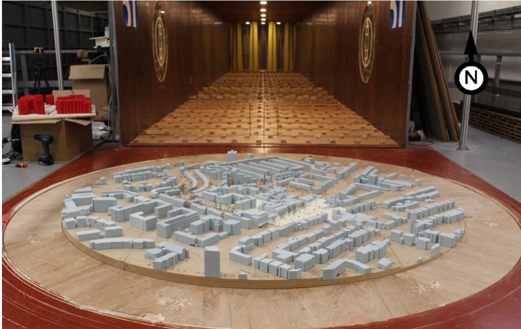
Figure 11: Existing Site with Existing Landscaping and Existing Surrounding Buildings (Configuration 1) – View in the Wind Tunnel (from the south)
