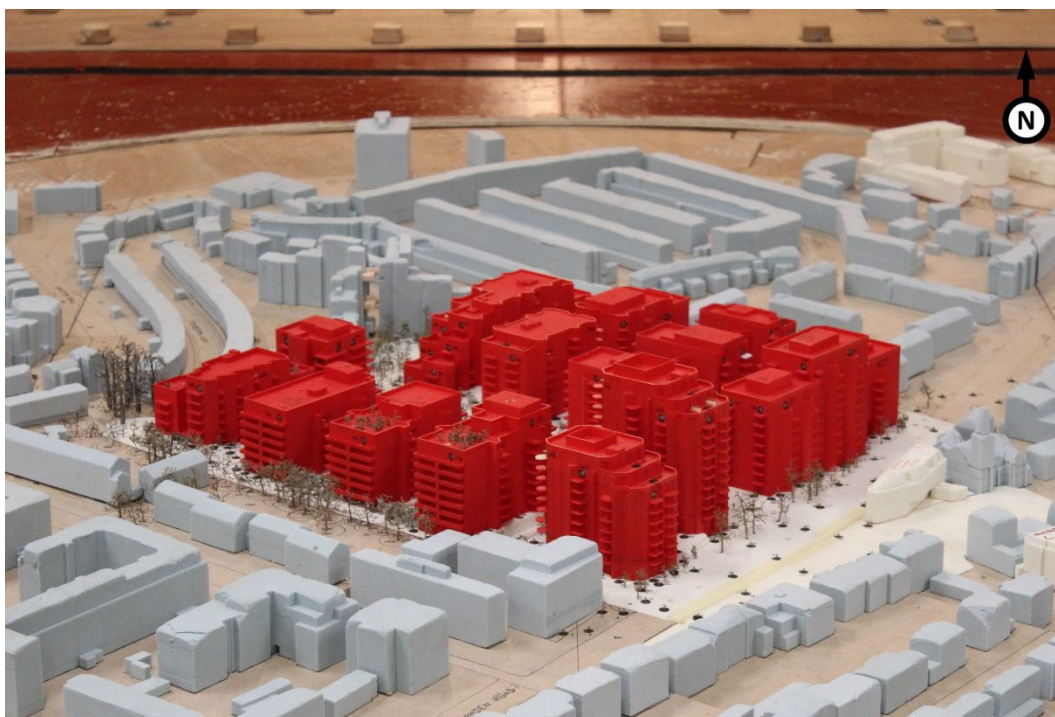
Figure 14: The Development with existing and proposed landscaping and cumulative schemes plus proposed mitigation measures (Configuration 6) – View in the Wind Tunnel (from the south)
