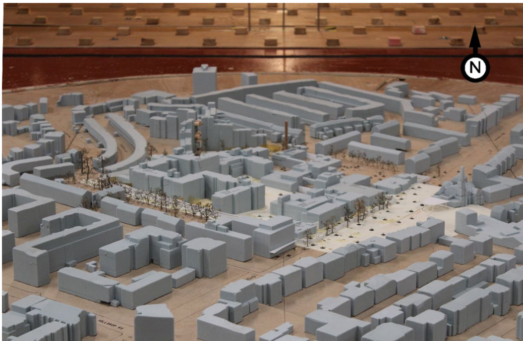
Figure 12: Existing Site with Existing Landscaping and Existing Surrounding Buildings (Configuration 1) – View in the Wind Tunnel (from the south)
