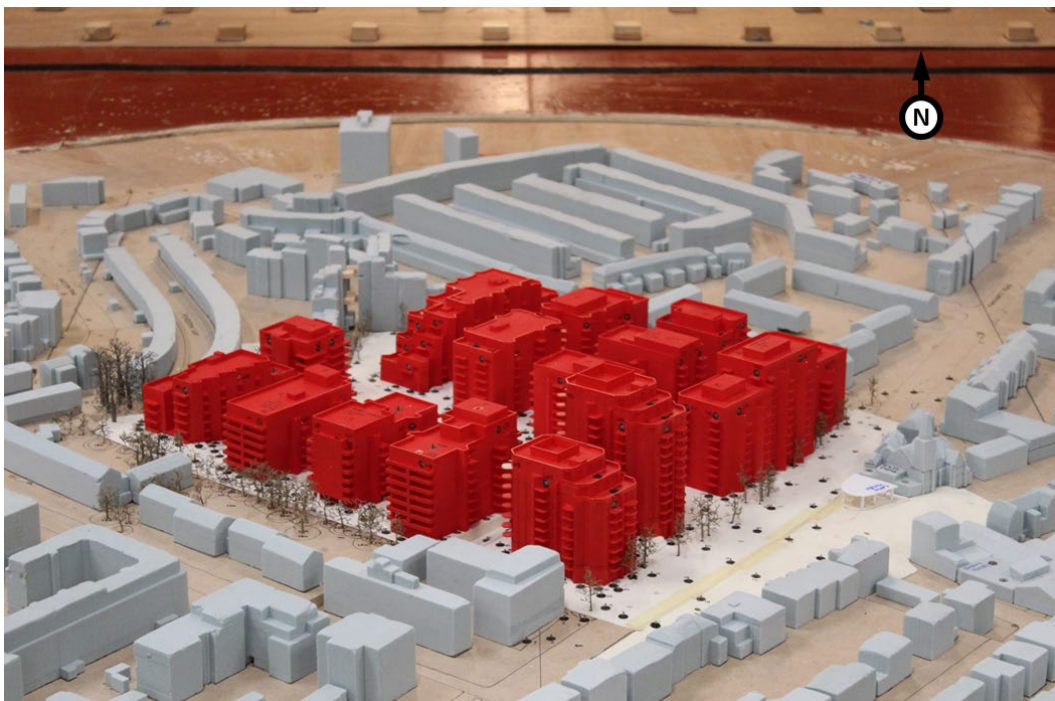
Figure 6: The Development with existing landscaping and existing surrounding (Configuration 2) – View in the Wind Tunnel (from the south)
