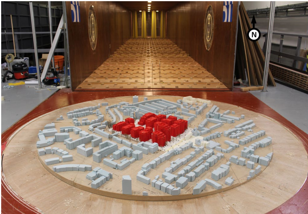
Figure 9: The Development with existing landscaping and Cumulative Schemes (Configuration 4) – View in the Wind Tunnel (from the south)
