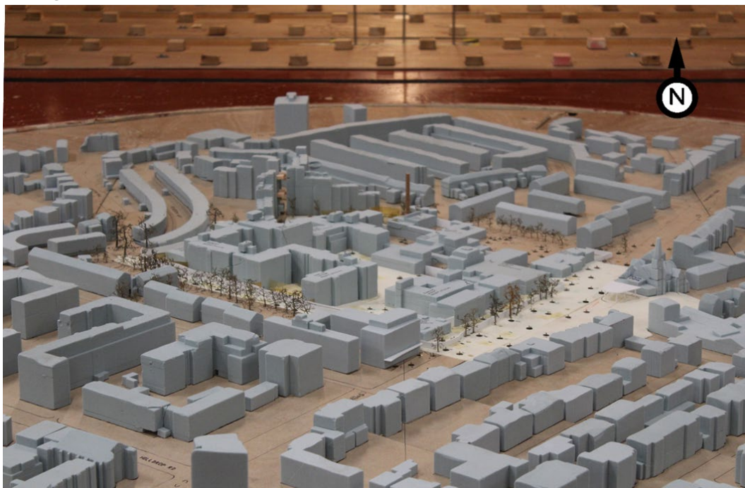
Figure 4: Existing Site with existing landscaping and existing surrounding buildings (Configuration 1) – View in the Wind Tunnel (from the south)
