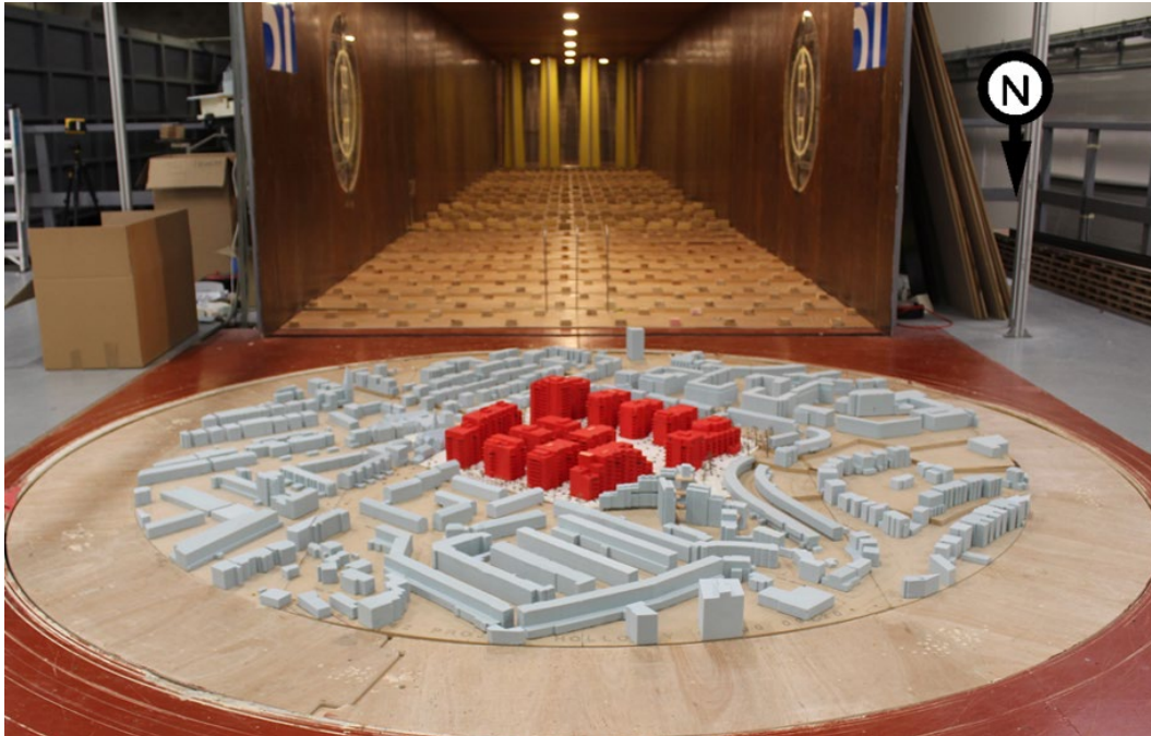
Figure 13: Proposed Development with Existing Landscaping and Existing Surrounding Buildings (Configuration 2) - View in the Wind Tunnel (from the north)
