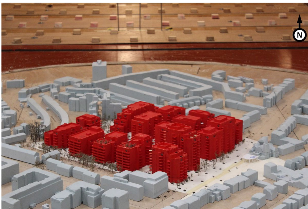
Figure 12: The Development with existing and proposed landscaping and existing surrounding buildings plus proposed mitigation measures (Configuration 5) – View in the Wind Tunnel (from the south)
