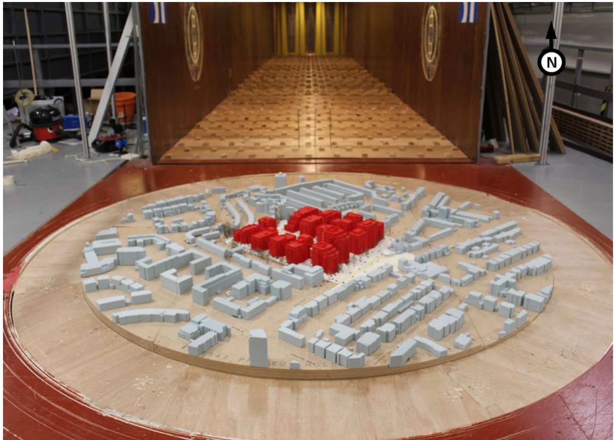
Figure 1: Image of the Development with existing landscaping and existing surrounding buildings (View in the wind tunnel from the south)
