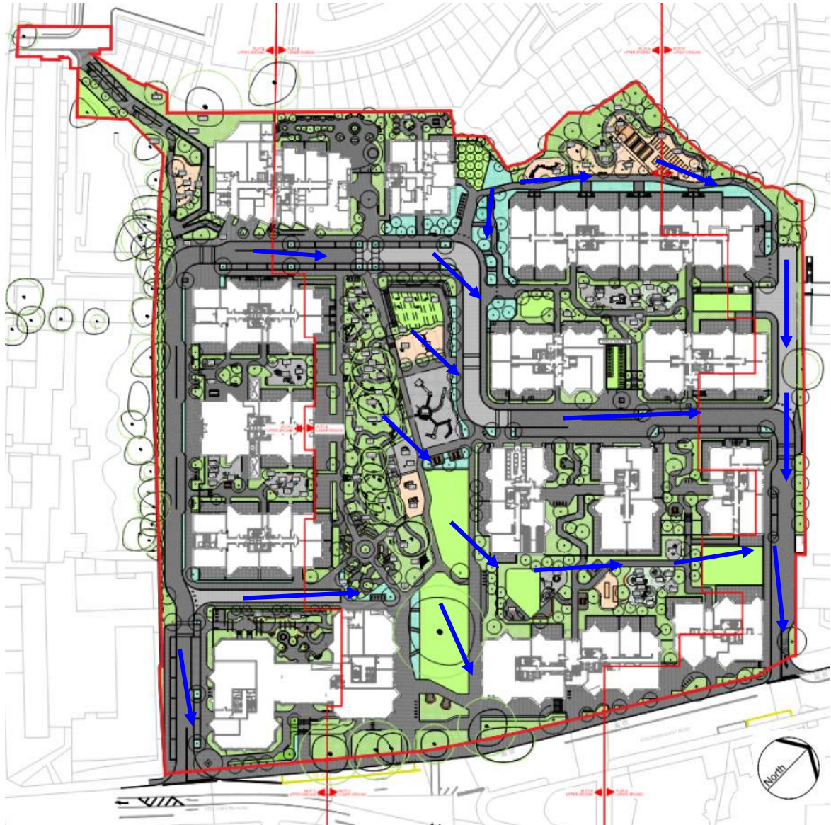
Figure 5: Exceedance flood flow routing
