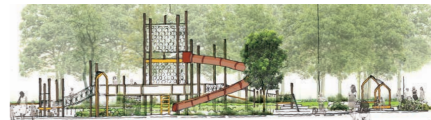
CUSTOM PLAY TOWER WITH SLIDES, SWING BRIDGES, CLIMBING NETS, HIGH ROPES COURSE, HAND GRIPS AND CLIMBABLE MESH, AND FEATURE SLIDES
