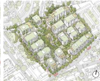
July 2021 Further iteration of the previous approach which further reduces the grain by breaking up the longer buildings into smaller building improving aspect and internal light levels.
