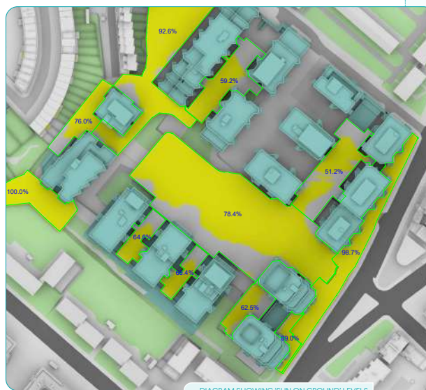
DIAGRAM SHOWING 'SUN ON GROUND' LEVELS
