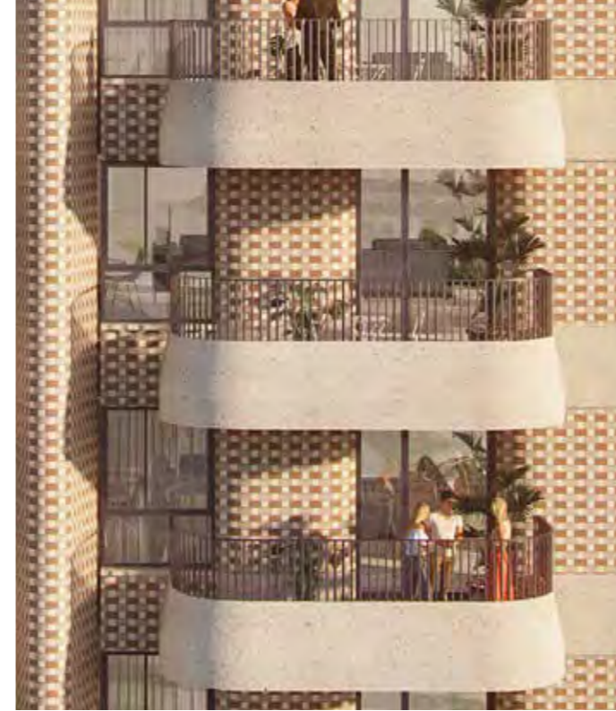
● Deeper concrete balconies with metal handrail
