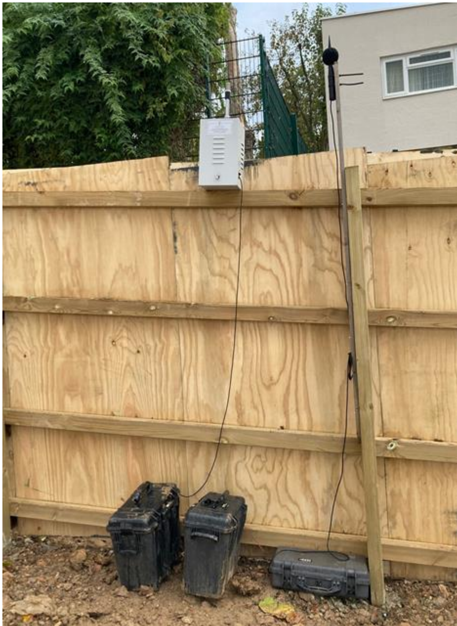
Location 2 – Dust, Noise and Vibration – northern boundary facing residential uses on Penderyn Way
