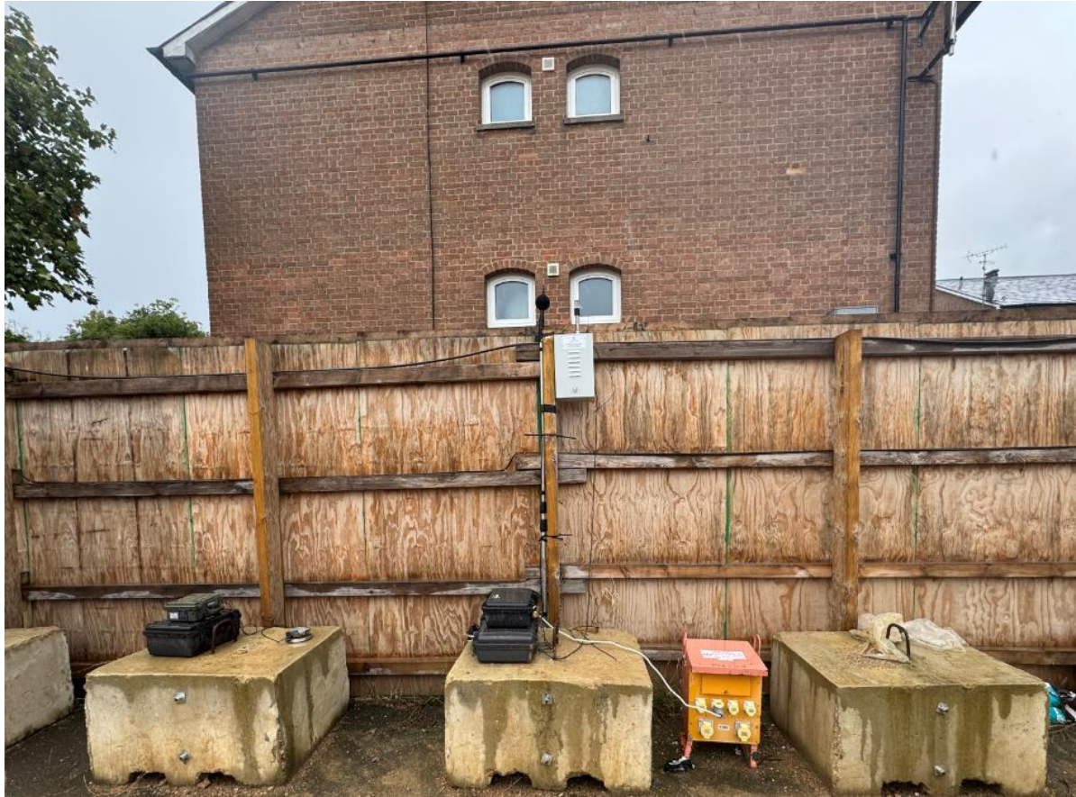
Location 3 – Dust, Noise and Vibration – northeastern boundary facing residential uses within Holloway Estate
