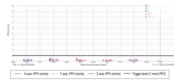
3.12 There was 100% data coverage at Location 4 for the monitoring period covered by this report. There were no exceedances of the project vibration trigger level of 1 mm/s PPV as shown in the raw data and graph above. Furthermore, the project team have confirmed that there are no active works in this areas of the site currently.
