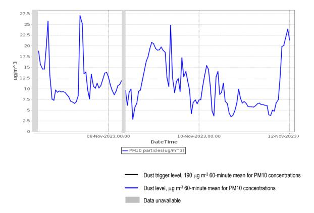
3.4 There was 93% data coverage at Location 3 for the monitoring period covered by this report. The only missing data occurred during Monday morning when the site team were swapping the depleted battery from the weekend. No exceedances of the project dust criteria of 190 micrograms per cubic meter were recorded during the monitoring period covered by this report.
