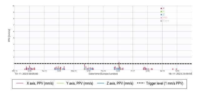
3.12 There was 100% data coverage at Location 4 for the monitoring period covered by this report. There was one exceedance of the project vibration trigger level of 1 mm/s PPV as shown in the raw data and graph above. The project team have confirmed that there are no active works in this areas of the site currently so this exceedance was likely due to non-construction related activities (i.e. weather related).
