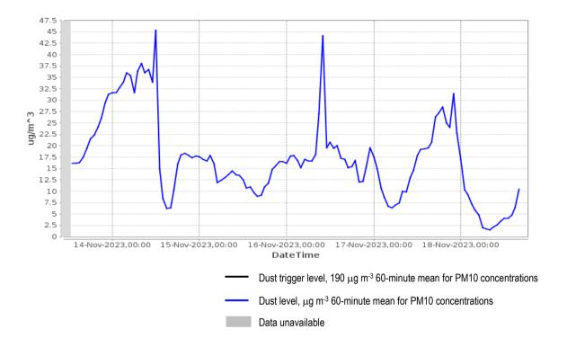
3.2 There was 91% data coverage at Location 1 for the monitoring period covered by this report. The only missing data occurred during Monday morning when the site team were swapping the depleted battery over from the weekend. No exceedances of the project dust limit of 190 micrograms per cubic meter were recorded during the period covered by this report.
