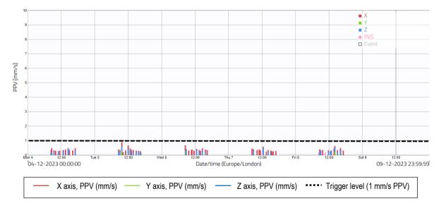
3.11 There was 100% data coverage at Location 4 for the monitoring period covered by this report. There were no exceedances of the project vibration trigger level of 1 mm/s PPV as shown in the raw data and graph above.
