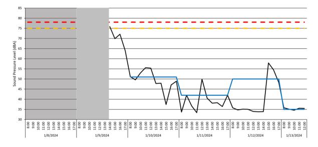
3.6 There was 71% data coverage at Location 2 for the monitoring period covered by this report. Cass Allen successfully replaced the faulty microphone cable on the 9<sup>th</sup> January. No exceedances of the project hourly noise criteria of 78 dB LAeq nor the daily project noise limit of 75 dB LAeq (0800-1800 hours) were recorded during the monitoring period covered by this report.
