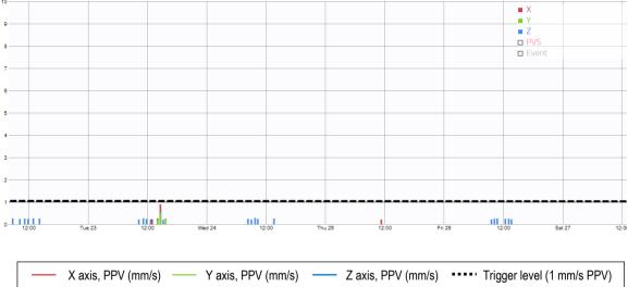
3.8 There was 100% data coverage at Location 1 for the monitoring period covered by this report. There were no exceedances of the project vibration trigger level of 1 mm/s PPV as shown in the raw data and graph above.
