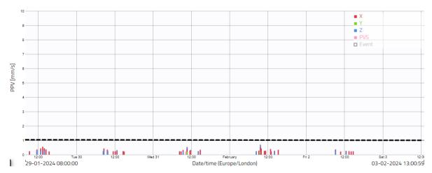
3.11 There was 100% data coverage at Location 4 for the monitoring period covered by this report. There were no exceedances of the project vibration trigger level of 1 mm/s PPV as shown in the raw data and graph above.
