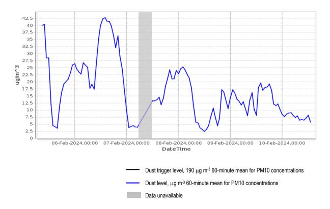
3.2 There was 93% data coverage at Location 1 for the monitoring period covered by this report. The monitor was offline for the first three working hours of Wednesday 7<sup>th</sup> February, before the battery change was completed. No exceedances of the project dust criteria of 190 micrograms per cubic meter were recorded during the monitoring period covered by this report.
