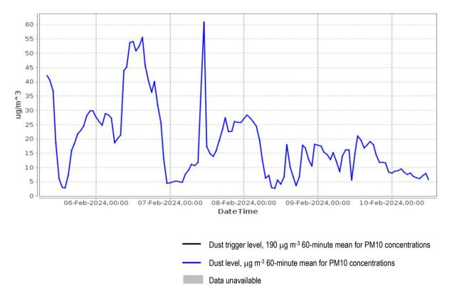
3.4 There was 100% data coverage at Location 3 for the monitoring period covered by this report. No exceedances of the project dust criteria of 190 micrograms per cubic meter were recorded during the monitoring period covered by this report.
