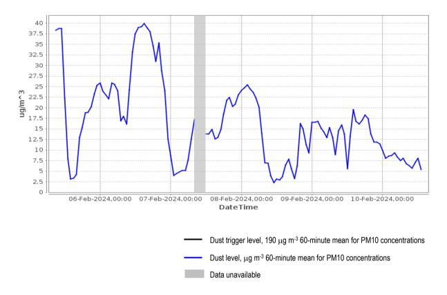
3.3 There was 93% data coverage at Location 2 during construction hours for the monitoring period covered by this report. The monitor was offline for the first three working hours of Wednesday 7<sup>th</sup> February, before the battery change was completed. No exceedances of the project dust criteria of 190 micrograms per cubic meter were recorded during the monitoring period covered by this report.
