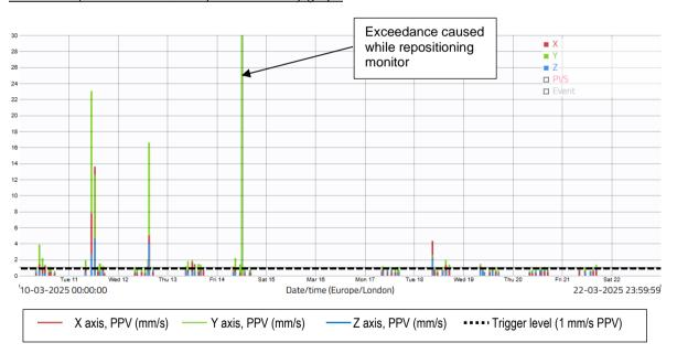
3.17 There was 100% data coverage at Location 2 during construction hours for the monitoring period covered by this report. There were 101 exceedances of the project vibration trigger level of 1.0 mm/s PPV, as shown in the raw data and graph above. Exceedances recorded on Friday 14<sup>th</sup> March between 12:00 and 12:40 can be discounted, which were caused by site personnel during a Cass Allen site visit, which took place at the time.
