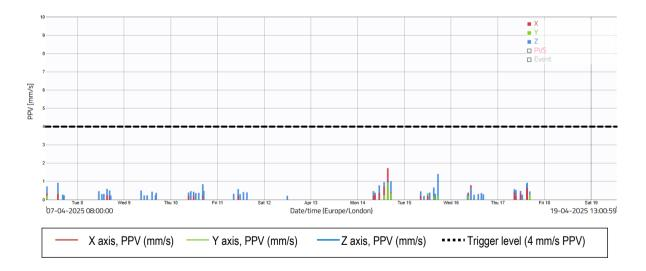
3.17 There was 100% data coverage at Location 3 during construction hours for the monitoring period covered by this report. There were no exceedances of the project vibration trigger level of 4.0 mm/s PPV, as shown in the raw data and graph above.
