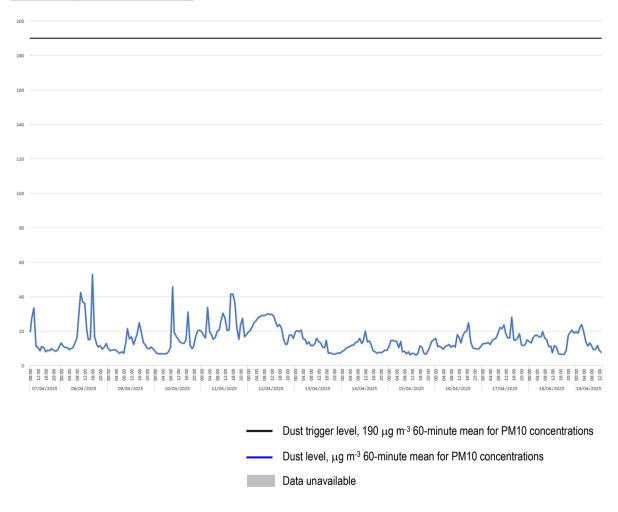
3.2 There was 100% data coverage during the monitoring period. There were no exceedances of the dust trigger of 190 μg m<sup>-3</sup> recorded at this location during construction hours.
