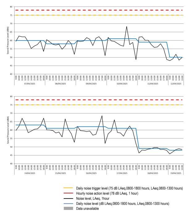
3.12 There was 100% data coverage at Location 3 during construction hours for the monitoring period covered by this report. There were no exceedances of the daily noise trigger level (75 dB LAeq,T) or the hourly noise action level (78 dB LAeq,1hr) during this monitoring period.
