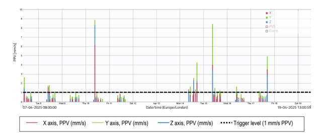
3.14 There was 100% data coverage at Location 2 during construction hours for the monitoring period covered by this report. There were 117 exceedances of the project vibration trigger level of 1.0 mm/s PPV, as shown in the raw data and graph above.
